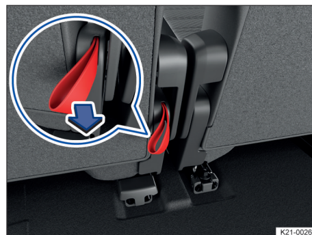
Fig. 3 Second row seats: loop for third row seat emergency exit function.
